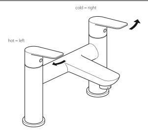
Moving the levers in the direction of the arrows will increase the flow of water.
