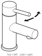
Moving the mixer lever upwards/downwards will increase/decrease the flow of water. Moving the mixer lever from right to left will increase the water temperature. Pull the vertical control rod up to close the waste outlet and push down to open.
