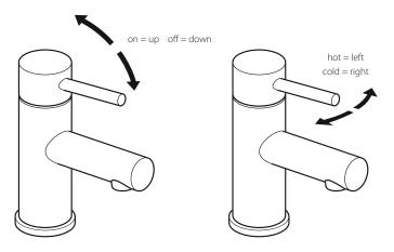
Moving the mixer lever upwards/downwards will increase/decrease the flow of water.
