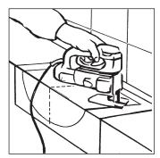
4 Using the preferred cutting tool, cut along the indicated line on the template whilst being careful not to cut on the outside of the indicated line.
