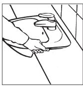
**9** Remove excess sealant from around the basin whilst making sure the basin is properly installed.
