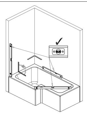
Verify screen location is level, plumb, and square. Check dimensions of bath to ensure proper fit of screen
