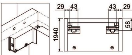
Fix Hanging plates (1) to the wall using suitable fixings (not supplied).
