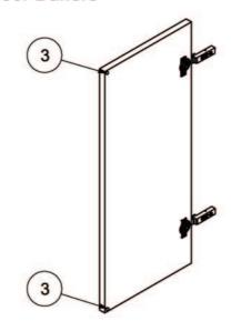
Position Door Buffers (3) at the top and bottom of each mounted door.
