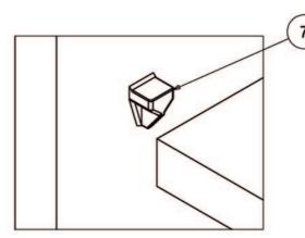
Select desired shelf position and insert Shelf Supports (7). Place the Shelf Panel on top of the Shelf Supports.
