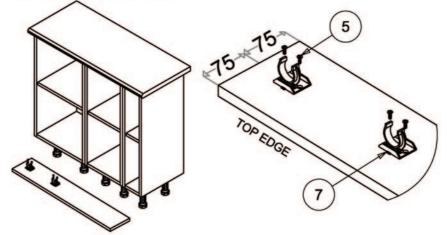
**Position Plinth Mounting** Brackets (7) 75mm from the top edge of the plinth and aline length ways with the cabinet legs. Attach using screw (5).
