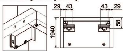
Fix Hanging plates (1) to the wall using suitable fixings (not supplied).
