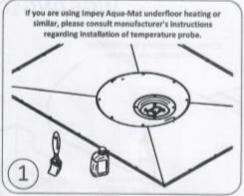
Ensure the surface is clean, dry, free from dust, grease, oil etc., all indentations should be filled and any protrusions struck off. Oily or greasy surfaces should be cleaned with a suitable cleaner, thoroughly rinsed then allowed to dry. Apply the primer to all porous surfaces.
