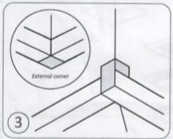
Using the 150mm jointing tape, line all the corners and wall/floor junctions so that the tape overlaps 75mm at the wall and 75mm onto the floor.
