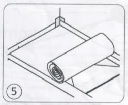
Measure and cut required length of Waterguard Membrane. Remove the release paper and carefully set into position - pressing firmly onto the jointing tape. Repeat steps 4 and 5 until the floor is covered.
