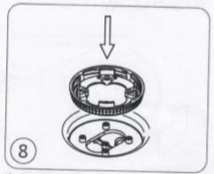
After the membrane is cut, the clamp can be gently pressed into place. Ensure the clamp is fully down before hand tightening the four clamp screws evenly.
