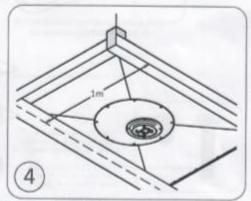
Measure Im (the width of the sheet of Waterguard Membrane) and mark a guide line for the jointing tape. Removing the release paper set the tape down so that the guide line runs along the centre of the tape.
