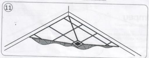
The installation of EasyFit Dec is now finished. Apply tiles to the whole area. If you are using large format tiles, they must be cut diagonally to follow the falls in the Dec, e.g. from the corners of the tiling frame to the corners of the Dec. in all cases the tiles must be laid to follow the falls/gradient of the Dec.
