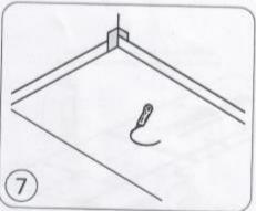
Locate the centre of the drain and cut a circular hole to 115mm diameter (central to the bowl). Care should be taken not to damage the drain when cutting the hole.
