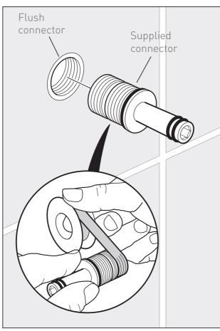
Slide the outlet over the connector until it touches the wall.
