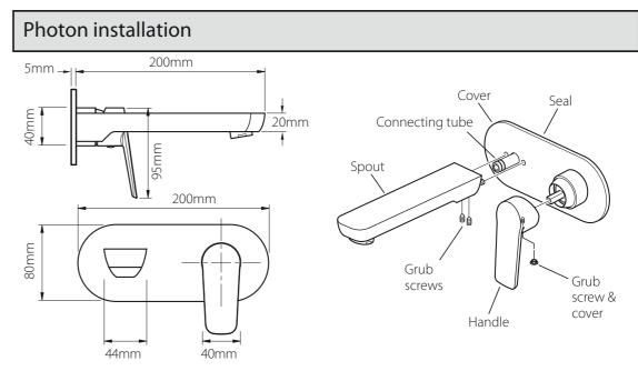
Remove the backing paper from the seal on the back of the cover. Slide the cover over the valve, push onto the wall until it makes contact. Carefully slide the control handle onto the valve and secure in position with the grub screw within the handle using the hexagonal key supplied, replace the screw cover. Push the spout over the connecting tube, secure using the grub screws on the underside. Apply a small bead of silicone around the plate to seal against the tile.
