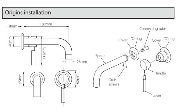
Slide the cover over the valve, push onto the wall until it makes contact. Carefully slide the control handle onto the valve and secure in position with the grub screw under the handle using the hexagonal key supplied, screw the lever onto the handle. Screw the spout into the cover. Push the spout over the connecting tube, secure using the grub screws on the underside.
