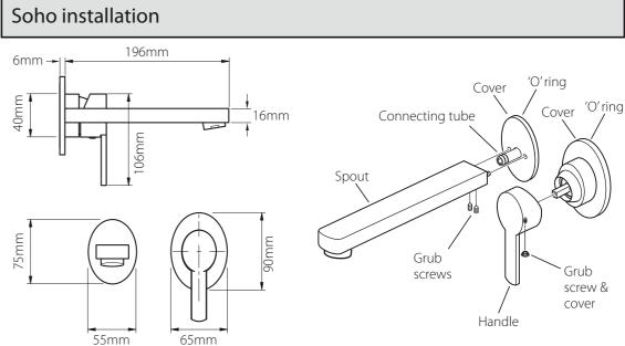
Slide the cover over the valve, push onto the wall until it makes contact. Carefully slide the control handle onto the valve and secure in position with the grub screw within the handle using the hexagonal key supplied, replace the screw cover. Slide the cover over the connecting tube, Push the spout over the connecting tube, secure using the grub screws on the underside.
