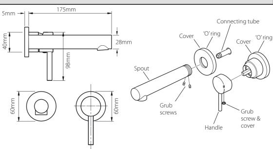
Slide the cover over the valve, push onto the wall until it makes contact. Carefully slide the control handle onto the valve and secure in position with the grub screw within the handle using the hexagonal key supplied, replace the screw cover. Screw the spout into the cover. Push the spout over the connecting tube, secure using the grub screws on the underside.
