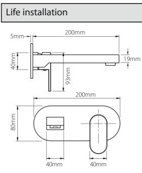
Remove the backing paper from the seal on the back of the cover. Slide the cover over the valve, push onto the wall until it makes contact. Carefully slide the control handle onto the valve and secure in position with the grub screw within the handle using the hexagonal key supplied, replace the screw cover. Push the spout over the connecting tube, secure using the grub screws on the underside. Apply a small bead of silicone around the plate to seal against the tile.
