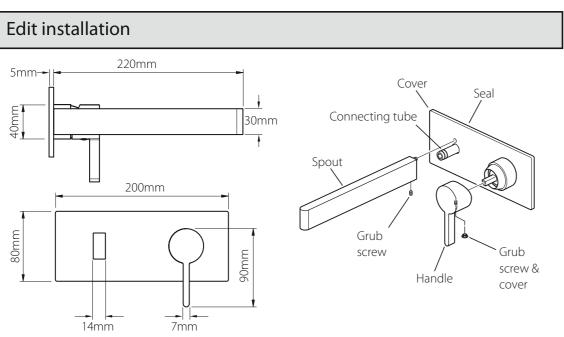
Remove the backing paper from the seal on the back of the cover. Slide the cover over the valve, push onto the wall until it makes contact.
