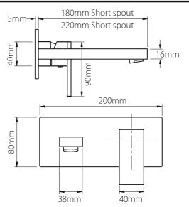
Remove the backing paper from the seal on the back of the cover. Slide the cover over the valve, push onto the wall until it makes contact. Carefully slide the control handle onto the valve and secure in position with the grub screw within the handle using the hexagonal key supplied, replace the screw cover. Push the spout over the connecting tube, secure using the grub screws on the underside. Apply a small bead of silicone around the plate to seal against the tile.
