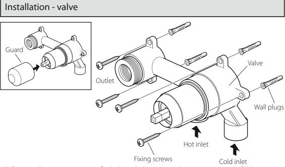
Before installing your new mixer, flush through the pipe work to ensure removal of debris, turn off the water supply.
