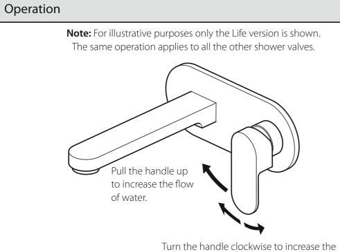
Turn the handle clockwise to increase the temperature and anti-clockwise to decrease the temperature.
