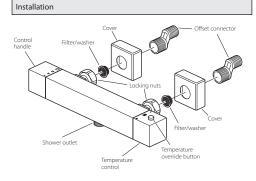
Before installing your new mixer, flush through the pipe work to ensure removal of debris, turn off the water supply Warning! Please check for any hidden cables and pipes before drilling holes in the
