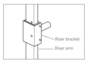
Carefully push the riser arm into the riser, the seals have been pre-greased to help the two slide together.
