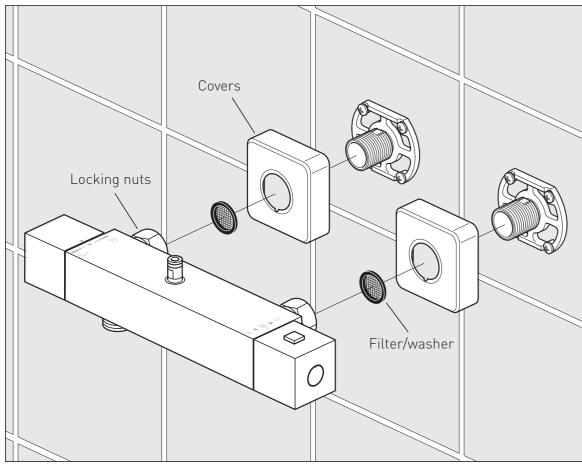
Screw the covers on each offset connector. Place a rubber filter/washer in each of the locking nuts on the valve and screw onto the connectors.
