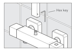
Make sure that the riser is vertical and secure in position using the grub screw on the top of the wall bracket.
