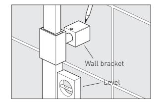
**Warning!** Please check for any hidden cables and pipes before drilling holes in the wall.
