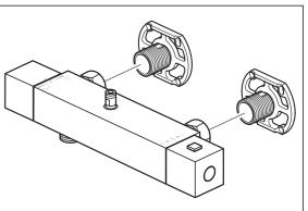
Position the valve making sure it is level and mark the position of the 4 screw holes in each connector.
