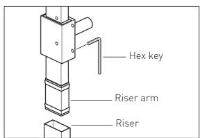
Slide the wall bracket on the riser bracket.
