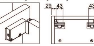
Fix Hanging plates (1) to the wall using suitable fixings (not supplied).
