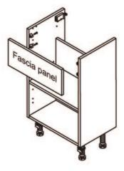
Attach the fascia panel using screws (8), brackets pre-fitted to cabinet side panels.
