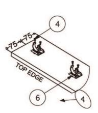
Position Plinth Mounting Brackets (6) 75mm from the top edge of the plinth and aline length ways with the cabinet legs. Attach using screw (4).
