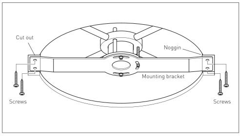
Position the mounting bracket and secure in place with 4 suitable screws, ensuring it is level.
