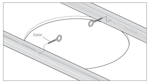
Securely screw the two eyelets into the ceiling joists/support.
