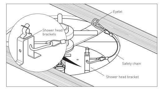
Attach the two easy clip safety chains. Clip one end of the safety chain to the eyelet and the other end into one of the holes on the shower head bracket. Repeat for the other side.
