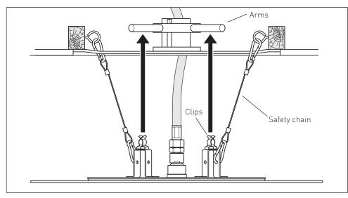
Align the clips directly below the arms, push the shower head until the clips snap into position.
