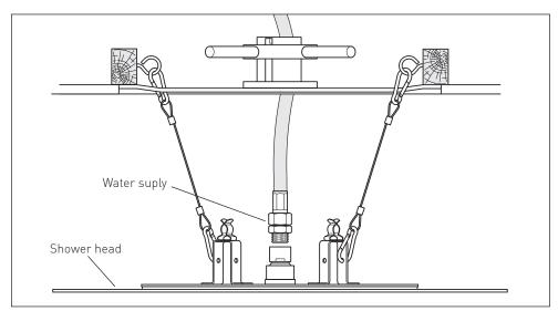
Using a flexible pipe connect the water supply to the shower head. Turn on flow and check for leaks.
