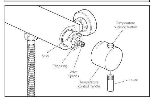
The valve has been factory set under balance pressures and hot water supply at 65° C. When your specific operating conditions are significantly different from the above, the temperature of the water may vary from the setting.
