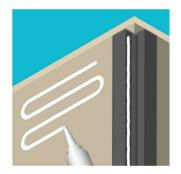
7. Place 3mm high spacers along the back +edge of the shower tray to create a 3mm clear gap at the panel base to be filled with sealant later.
