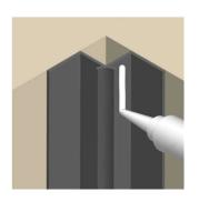
**6.** Apply adhesive to the wall in a series of waves from top to bottom of the area where the panel will be affixed.
