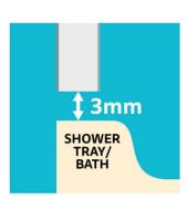
8. Position the panel above the 3mm spacers and slide into the internal trim recess/previous panel with your grooved edge exposed for your next panel. The sealant should envelope the
