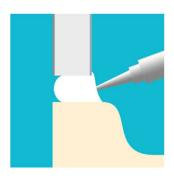
11. Cut-outs for shower heads and the like require an expansion gap of at least 3 mm. After fitting the boards these gaps must be filled with sealant.
