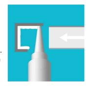
5. Apply a continuous bead of sealant into one recess of the internal trim. When fitting a second panel, apply a continuous bead of sealant into the T&G Profile before connecting panels
