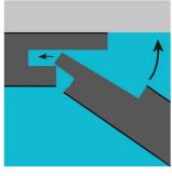
located onto the channel with the panel top edges flush. Rotate the panel onto the wall
