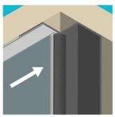
panel. Wipe away excess sealant. Apply even pressure across the panel face to ensure sound contact of the adhesive on the reverse of the panels.
