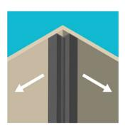
**2.** Apply a continuous bead of adhesive to the reverse of the internal trim and fix in position. Use a spirit level to ensure it is plumb.
